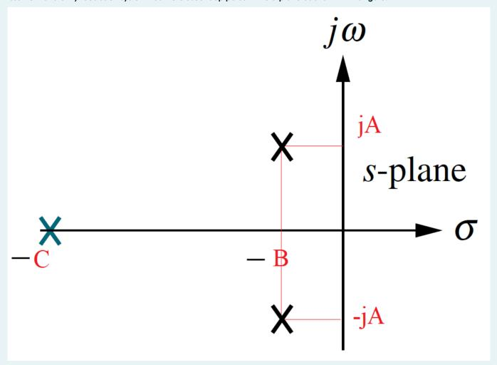
the the closed loop system has a unity DC gain, and If the value of A is 36, the value of B is 3 and the value of C is 30. Then, the EXACT closed-loop Transfer function of the system is:
